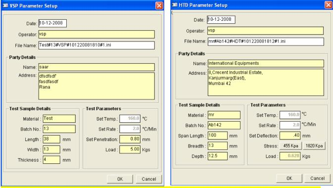
IN CASE OF VSP – 1KG OR 5 KG LOAD CAN BE DIRECTLY USED / IN CASE OF HDT YOU REQUIRE LOAD CALCULATION AS PER THE FORMULA WHERE BY YOU EITHER SELECT 455KPA OR 1820 KPA. AS YOU CAN SEE IN HDT SCREEN ABOVE THE IF YOU CLICK ON 455 KPA OR 1820 KPA DIRECTLY OUR SOFTWARE WILL CALCULATE THE LOAD AND SHOW IN THE BOTTOM LOAD WINDOW – WHICH CA BE DIRECTLY LOADED ON TEST ESSEMBLY.
