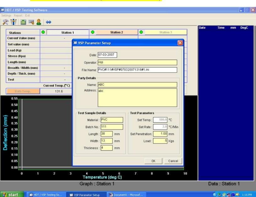
MAIN SCREEN DISPLAY WHEN TEST WILL RUN (RIGHT SIDE IT WILL SHOW SECOND TO SECOND DATA CAPTURING AND ON GRAPH IT WILL SHOW ACTUAL GRAPH, UP IT WILL SHOW SET DATA FOR BOTH THE TESTS BY USER
